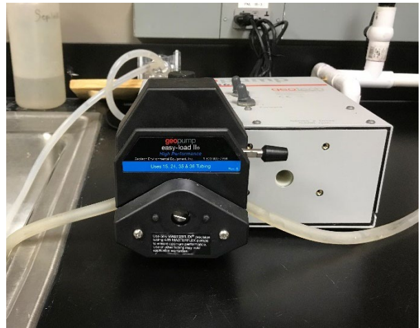
Figure 2. (Left) Example of how to load tubing into peristaltic pump with quick-release lever open. (Right) Once tubing is loaded, close the quick-release lever.
