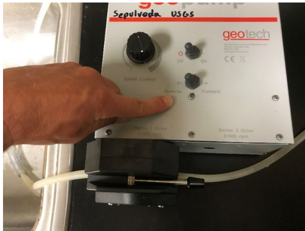
Figure 3. Set the direction of the pump (forward or reverse). In this photo, I am pulling water from the sample (on the right) and spilling the water in the sink (on the left); so, the pump is set in "Reverse".
